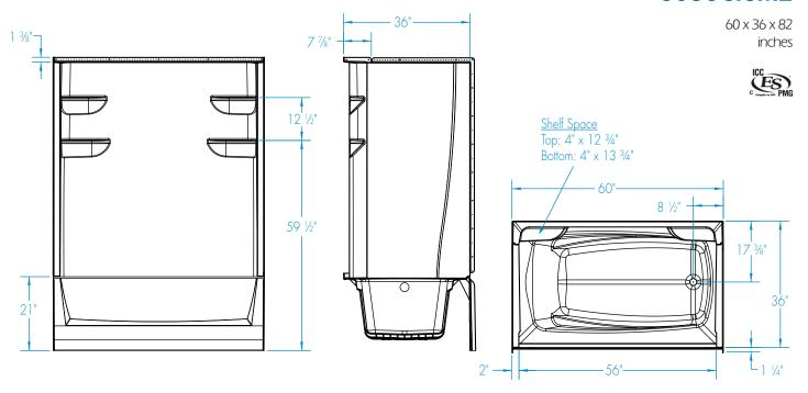
Assembled Model Components: 6036CTML (Base) or 6036CTMR (Base), 6062CBW2 (Back Wall), 2462CSW (Side Walls)
