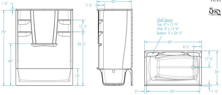
Assembled Model Components: 6036CTL (Base) or 6036CTR (Base), 6062CBW (Back Wall), 2462CSW (Side Walls)
