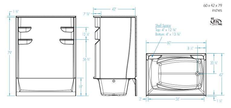
Assembled Model Components: 6042CTL (Base) or 6042CTR (Base), 6062CBW2 (Back Wall), 3562CSW (Side Walls)
