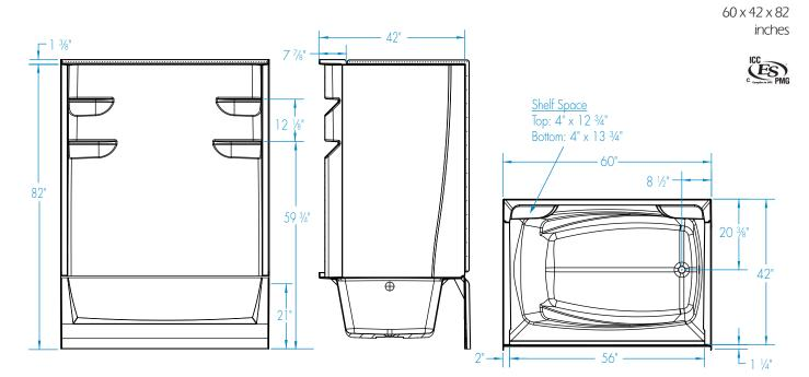
Assembled Model Components: 6042CTML (Base) or 6042CTR (Base), 6062CBW2 (Back Wall), 3562CSW (Side Walls) Age-In-Place Assembled Model Components: 6042CTML (Base) or 6042CTMR (Base), 6062CBW2A (Back Wall), 3562CSWA (Side Walls)
