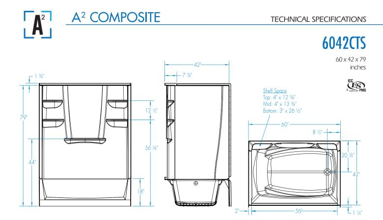
Assembled Model Components: 6042CTL (Base) or 6042CTR (Base), 6062CBW (Back Wall), 3562CSW (Side Walls)
