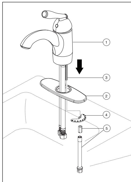
**SHUT OFF WATER SUPPLIES.** Position faucet (1) with single or three hole escutcheon (2) and baseplate (3) or gasket (3) on sink, studs (4) must pass through the holes on escutcheon (2) and baseplate (3). **Option:** If surface of sink is uneven, use silicone under the baseplate or gasket. Place metal bracket (5) over mounting stud (4) under sink. Secure with mounting nut & wrench (6).
