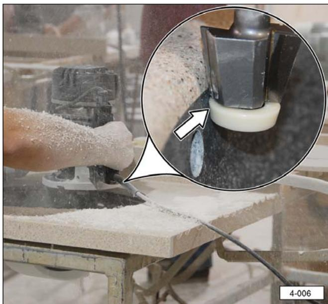
**Note:** Marks on the sink caused by the router bit bearing will be removed during the sanding process in a later section.
