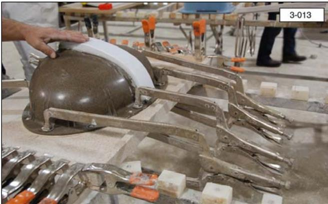
14. Once the sink is securely clamped in place, carefully remove one of the two screws from the rim of the sink, then retighten that screw. Repeat for the second rim screw. This will allow the clamps to apply full pressure to the sink rim, without having the sink slide out of position.
