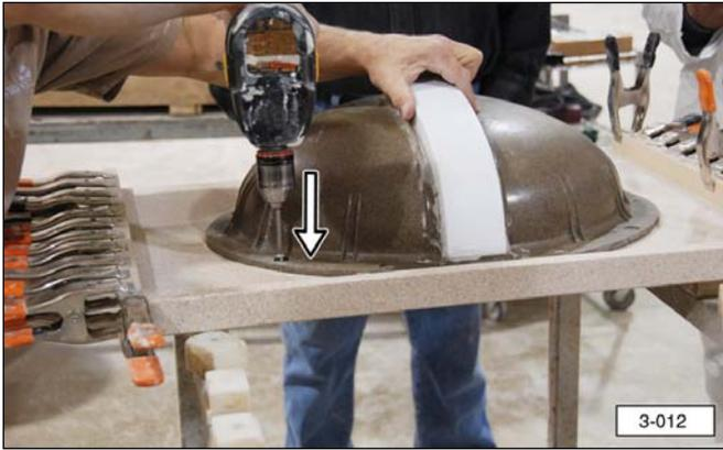
13. Clamp the sink in place using six to eight large deep-throat clamps applied to the rim of the sink and countertop, as shown.
