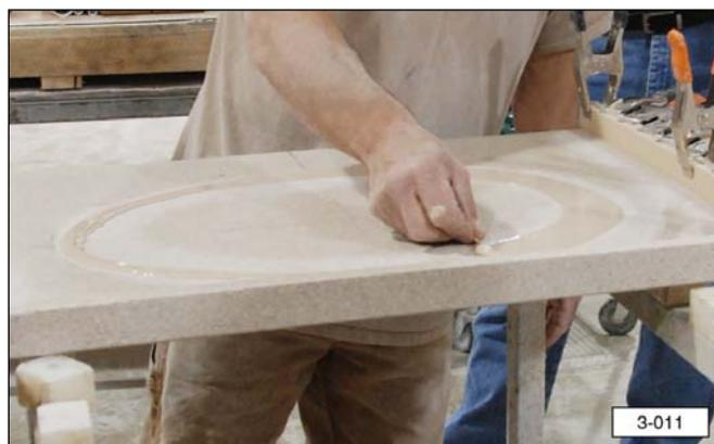
**Note:** Wear protective disposable gloves when working with the two-part acrylic adhesive. Remove excess acrylic adhesive with a flat blade putty knife. Clean up excessive acrylic adhesive with denatured alcohol and a clean cloth.
