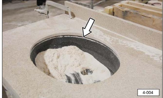
4. Inspect the seam between the sink and countertop, looking for any voids or cracks. If defects are found, the sink should be removed and reglued.
