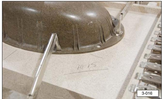
**Note:** Be very careful not to disturb the acrylic adhesive joints during the one hour cure time.
