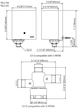
Thermostatic Mixing Valve (TLT10R)
