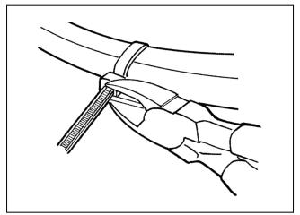
22. The plastic tie wraps provided can be used to hold the power cord and the air supply hose together.
