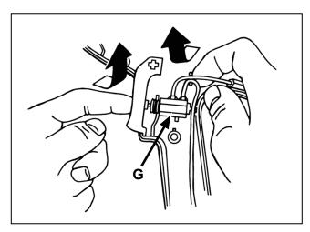
**8.** Pull the valve (G) out of the upper housing by lifting the tubing out of the notched ribs and lifting up on the trigger.
