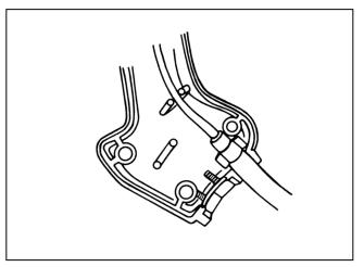
**14.** The proper position the lower portion of the air supply tubing and hose is shown above. These components will not stay in this position and must be held when the housings are mated in step 16.
