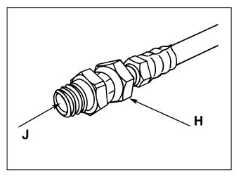
**10.** Remove the coupler filter (H) from the end of the faulty air supply line and install it on the end of the replacement air supply line.
