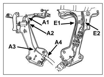
**15.** Check the locations indicated by arrows above to make sure all components are positioned properly.
