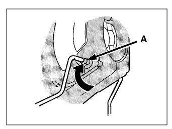
**20.** Pull the other end of the wirestand just enough to go over the edge of the applicator and position it into the pivot hole (A). The spring action of the wirestand will pull itself down into place.
