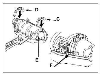
7. If the front standoff (C) or the rear standoff (D) is dislodged in any way, replace them on the heat tube (E). Upper and lower sets of standoffs should be in contact with no visible gaps between them at all four locations (F).
