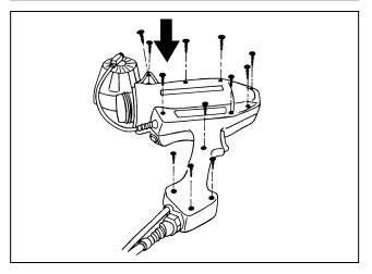
**18.** Recheck proper fit and alignment between the housing halves and make sure the trigger pivots freely.
