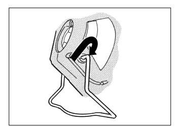
**21.** Pull the first end of the wirestand – from step 19 – out of the recess and position it over its pivot hole. The spring action of the wirestand will pull itself down into place.
