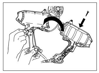
**16.** Hold trigger and the air hose in position in the upper housing and lift and turn the upper housing over onto the lower housing. Crossing the hands as shown will make it easier to hold the components in position while turning the housing over.
