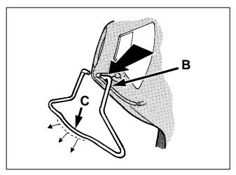
**19.** Hold the wirestand so the rounded part (C) curves away from the applicator and temporarily hook one end of the wirestand so the end rests down in the bottom of the recess (B) as shown.
