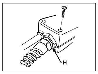
17. Separate the housing halves at the bottom of the handle just enough to adjust the position of the power cord strain relief. The hex (H) should be aligned and fully engaged with the matching hex-shaped recess in the housings. If necessary, rotate the strain relief hex one flat in either direction to obtain good fit.
