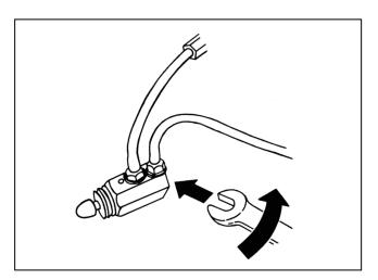
**9.** Use a 1/4 in. open end wrench and remove the brass fitting that connects the air supply tubing to the valve.
