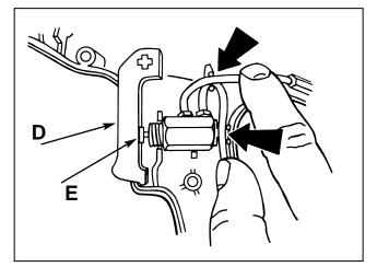
**13.** Place the valve in position and press the tubing down into the grooved ribs as shown. The tubing on the replacement air supply line should be underneath the tubing that connects to the endcap.
