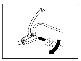
**12.** Use a 1/4 in. open end wrench and tighten the fitting to the valve securely.
