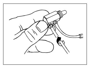
**11.** Attach the replacement air supply line to the valve by holding the brass fitting in position and turning the air hose clockwise.
