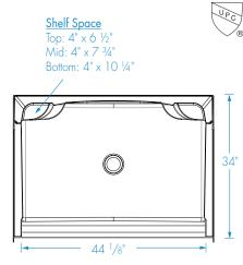
Assembled Model Components: 4834CPAN (Base), 4874CBW (Back Wall), 2774CSW (Side Walls)
