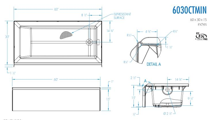
FEATURES Dimensional Tolerance ± %". Dimensions needed for site preparation should be measured from the unit. Manufacturer assumes no responsibility for preparatory work.
