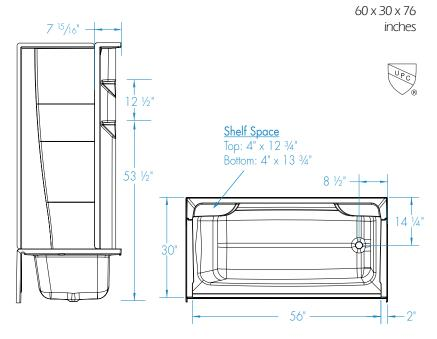
Assembled Model Components: 6030CTL (Base) or 6030CTR (Base), 6062CBW2 (Back Wall), 2462CSW (Side Walls)
