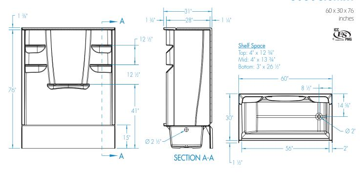
Assembled Model Components: 6030CTMINL (Base) or 6030CTMINR (Base), 6062CBW (Back Wall), 2462CSW (Side Walls)
