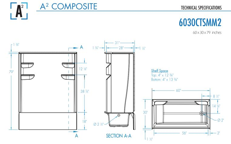
FEATURES Dimensional Tolerance ± %". Dimensions needed for site preparation should be measured from the unit. Manufacturer assumes no responsibility for preparatory work.
