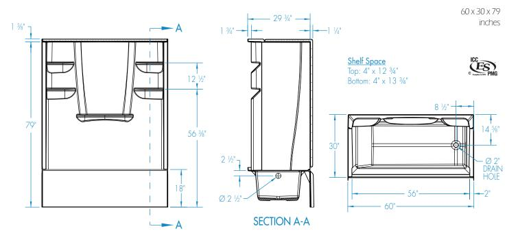
Assembled Model Components: 6030CTMML (Base) or 6030CTMMR (Base), 6062CBW (Back Wall), 2462CSW (Side Walls)
