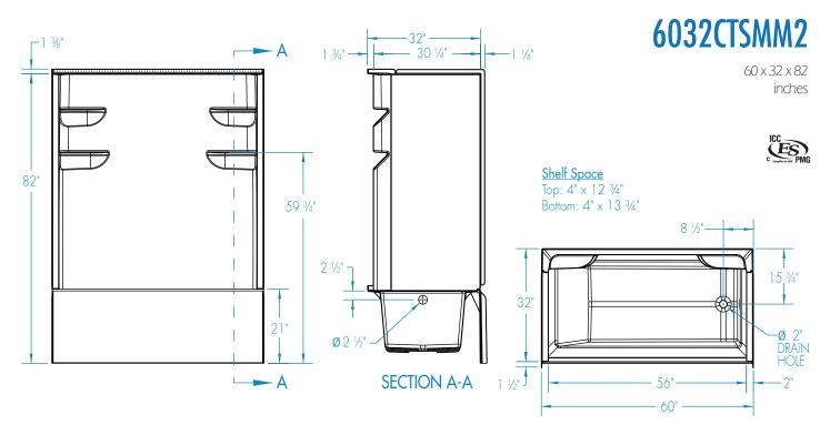
Assembled Model Components: 6032CTMML (Base) or 6032CTMMR (Base), 6062CBW2 (Back Wall), 2562CSW (Side Walls)
