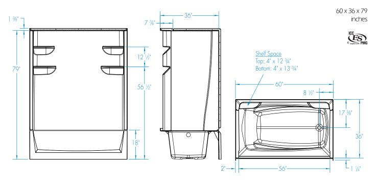
Assembled Model Components: 6036CTL (Base) or 6036CTR (Base), 6062CBW2 (Back Wall), 2462CSW (Side Walls)
