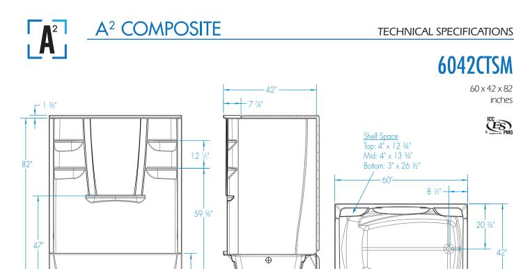
Assembled Model Components: 6042CTML (Base) or 6042CTMR (Base), 6062CBW (Back Wall), 3562CSW (Side Walls) Age-In-Place Assembled Model Components: 6042CTML (Base) or 6042CTMR (Base), 6062CBWA (Back Wall), 3562CSWA (Side Walls)
