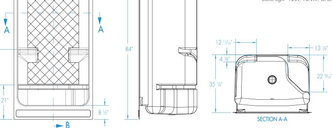
FEATURES lbs Dimensional Tolerance ± 3/8". Dimensions needed for site preparation should be measured from the unit. Aquatic assumes no responsibility for preparatory work.
