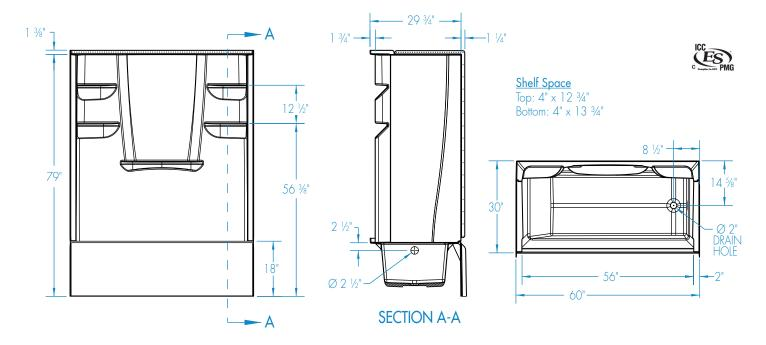
FEATURES Dimensional Tolerance ± 3/6". Dimensions needed for site preparation should be measured from the unit. Aquatic assumes no responsibility for preparatory work.
