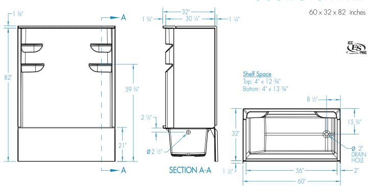
FEATURES (kg) Dimensional Tolerance ± %". Dimensions needed for site preparation should be measured from the unit. Aquatic assumes no responsibility for preparatory work.
