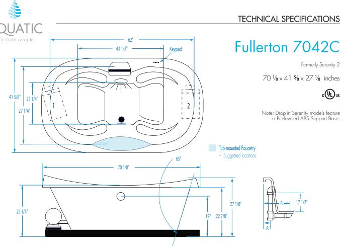
$\label{eq:FEATURES} \textbf{ Dimensional Tolerance} \pm 3/8 \text{''}. \textbf{ Dimensions needed for site preparation should be measured from the unit. Manufacturer assumes no responsibility for preparatory work.}$
