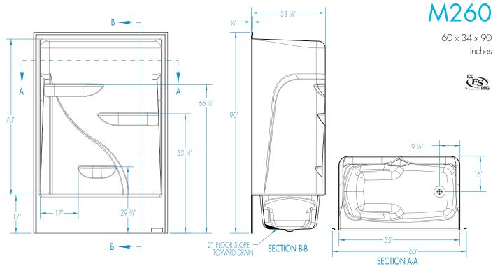
FEATURES lbs Dimensional Tolerance ± 3/8". Dimensions needed for site preparation should be measured from the unit. Aquatic assumes no responsibility for preparatory work.
