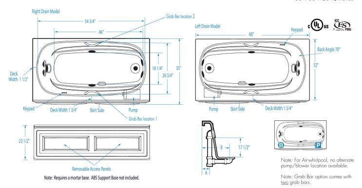
FEATURES | lbs (kg) | Dimensional Tolerance ± 3/8". Dimensions needed for site preparation should be measured from the unit. Aquatic assumes no responsibility for preparatory work.
