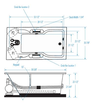
FEATURES Ibs (kg) Dimensional Tolerance ± 3/8". Dimensions needed for site preparation should be measured from the unit. Aquatic assumes no responsibility for preparatory work.
