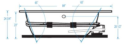
FEATURES Ibs (kg) Dimensional Tolerance ± 3/8". Dimensions needed for site preparation should be measured from the unit. Aquatic assumes no responsibility for preparatory work.
