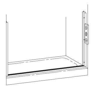
Run two beads of caulk inside the penciled marks on the tub rim.
