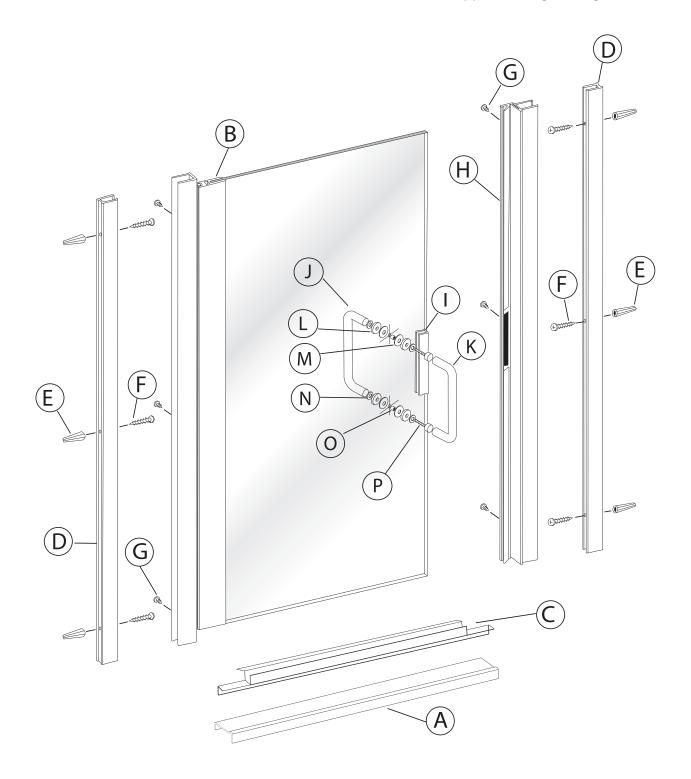
The Aquatic Shower Door is completely reversible and may be installed hinge-right or hinge-left. Refer to the illustration to determine the best hinge position for your installation. For maximum waterproofing, the hinge jamb should always be opposite the shower head. The following instructions depict a hinge-left installation.
