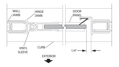
Inside the shower enclosure, using the pencil marks on the wall jambs from the previous step, drill two 1/8" holes through the hinge jamb of the door panel assembly and into the wall jamb 3/8" to 3/4" from the wall and approximately 1" down from the top and up from the bottom of the hinge jamb. Drill a third hole centered between the first two.
