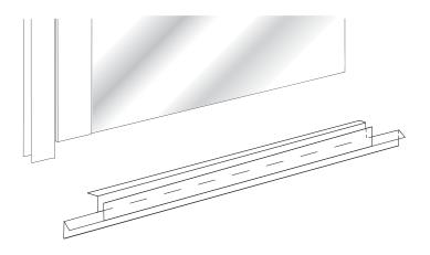
11 Align the clear bottom sweep to the bottom of the door with the deflector lip on the inside of the shower door. Mark the strike side of the bottom sweep even with the strike edge of the door.
