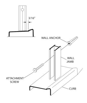
4 Measure the finished wall-to-wall opening at the top and botom of the wall jambs. Note the smaller dimension. (see bottom left illustration)
