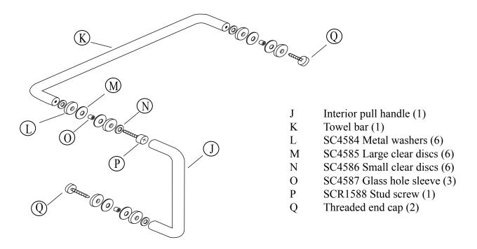
STEP 1 Take the stud head screw and sleeve a 1 1/4" washer on it. Now take both end caps with a threaded stud protruding and sleeve a 1 1/4" washer on them. Sleeve a clear gasket on each of the screws.
