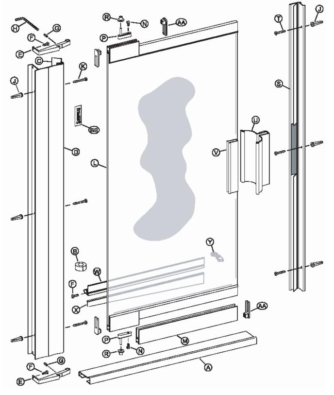
The Aquatic Shower Door is completely reversible and may be installed pivot-right or pivot-left. Refer to the illustration to determine the correct position for your installation. For maximum waterproofing, the pivot jamb should always be opposite the shower head. These instructions depict a pivot-left installation.
