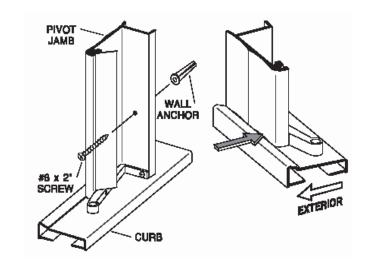
Replace the pivot jamb and attach to the wall with three  $\#8 \times 2$ " truss head screws [K].
