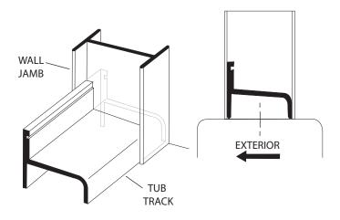
2 Using a level, plumb one wall jamb and mark the three hole locations on the wall with a pencil. Repeat this step for the other wall jamb. Remove all parts and drill the holes.
