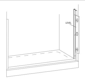
**CAUTION:** The bottom track should never be screwed to the threshold.
