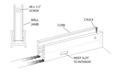
Place the setting blocks [H] in the curb assembly as shown to support the two fixed glass panels [J]. The setting blocks should be positioned approximately 3" from each corner of the panels. It should rest on the setting blocks and be engaged approximately 1/2" into the wall jamb [E]. A strip of masking tape 1/2" from each vertical edge of the glass will aid alignment.
