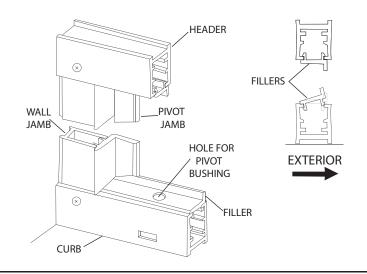
Pull the bottom end of the pivot jamb [P] tight to the curb filler [S] and plumb the jamb. Drill two 1/8" holes thru the pivot jamb and into the wall jamb [E] 3/8" to 3/4"from the wall and approximately 1/4" vertically from the ends of the jamb. Drill a third hole centered between the first two, then enlarge the outer holes with a 3/16" drill for clearance on the self-tapping screws. Attach the pivot jamb permanently with three #8 x 1/4" truss head screws [C].
