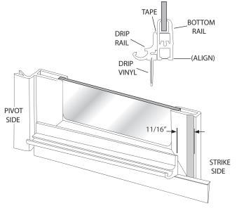
Adjust the drip vinyl [V] by sliding it left or right until it almost touches the curb. Trim the vinyl (flush with the pivot end and notch 1/4" longer than the drip rail as shown on the strike end).
