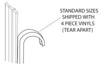
Cut eight pieces of the smaller vinyl [GG] 1" longer than the vertical opening (to prevent gapping from shrinkage) and trim the ends on a  $45^{\circ}$  angle. Using the masking tape guides, center the first glass panel [J] in the frame. Cut four short (1"-2") pieces of the small vinyl and press into the jamb and post on each side to hold the glass temporarily.
