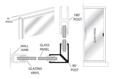
Cut eight pieces of the larger vinyl [HH] 1/2" longer than the horizontal opening and trim the ends on a 45° angle. Install the top exterior vinyl starting at both ends and working toward the middle. Be careful not to stretch the vinyl.
