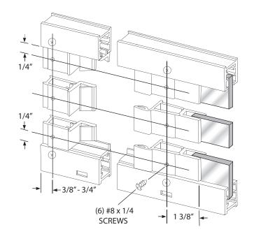
Clean the bottom door rail and the drip rail thoroughly with rubbing alcohol to ensure proper adhesion. Unroll the double stick tape [X] and carefully apply it to the back of the drip rail (do not peel the tape backing yet).
