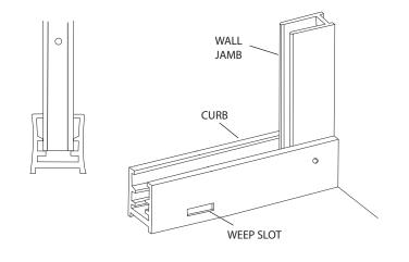
Wipe the shower walls and sill, the curb [A] and the wall jambs [B] with a clean, dry cloth to remove any dust or debris. Apply a 1/4" bead of caulk along the inside of both of the pencil lines marked in Step #2. Carefully replace the curb in the exact position marked. Caulk the inside of the curb ends where they meet the wall. Replace both wall jambs and attach to the walls with six #8 x 1 1/2" truss head screws [D].
