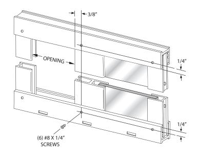
Orient the door to the opening (either hinge right Or hinge left). Place the door in the opening with the door hinge over the wall jamb or post. Carefully hold the door in the opening (in the open position) and don't let go of the door. Place the top filler to the under side of the header WITH THE RAISED LIP TO THE EXTERIOR and snap it into place.
