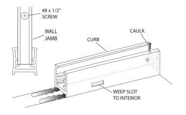
Place two setting blocks [E] into the curb [A] to support the fixed glass panel [F]. Position the blocks 3" from each corner of the glass panel. Set the glass panel into place on the setting blocks and approximately 1/2" into the wall jamb [B]. A strip of masking tape 1/2" from each vertical edge of the glass will aid alignment.
