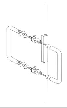
NOTE: The deflector [Q] is notched on both ends. To install deflector, determine if the door is hinge right or hinge left.
