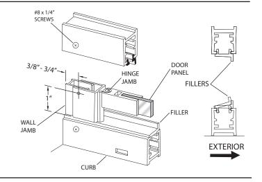
Pull the bottom end of the hinge jamb [L] tight to the curb filler [N] and plumb the jamb. Drill two 1/8" holes thru the hinge jamb and into the wall jamb [B] 3/8" to 3/4" from the wall and approximately 1/4" from the ends of the jamb. Drill a third hole centered between the first two, then enlarge the three outer holes with a 3/16" drill for clearance on the self-tapping screws. Attach the pivot jamb permanently with three #8 x 1/4" truss head screws [K].
