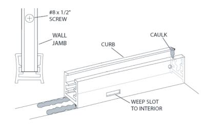
Place two setting blocks [E] into the curb [A] to support the fixed glass panel [F]. Position the blocks 3" from each corner of the glass panel. Set the glass panel into place on the setting blocks and approximately 1/2" into the wall jamb [B]. A strip a masking tape 1/2" from each vertical edge of the glass will aid alignment.
