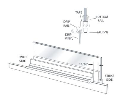
Adjust the drip vinyl [U] by sliding it left or right until it almost touches the curb. Trim the vinyl (flush with the pivot end and notch 1/2" longer than the drip rail as shown on the strike end). Secure it with one #6 x 3/8" truss head screw [EE] in the pivot end of the drip rail [S].
