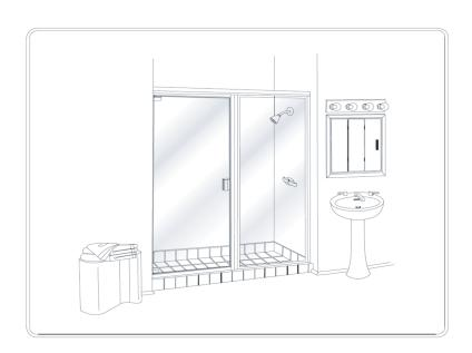
**MAINTENANCE:** Two primary materials are used to manufacture your new Aquatic enclosure: tempered glass and anodized aluminum. To assure a long lasting finish on the enclosure, wipe it down with a towel after each use. Never use a scouring agent to clean the aluminum.
