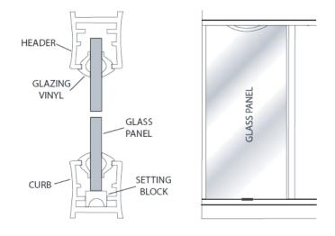
Carefully caulk the interior jamb-to-wall and curb-to-base joints. For appearance, you may wish to caulk the exterior joints as well. We recommend you wait twenty-four hours before the first shower to allow the caulking to cure properly.
