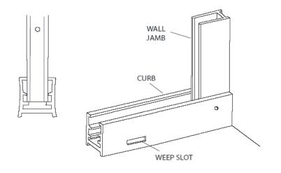
Wipe the shower walls and sill, curb [A] and wall jambs [B] with a clean, dry cloth to remove any dust or debris. Apply a 1/4" bead of caulk along the inside of both of the pencil lines marked in Step #2. Carefully replace the curb in the exact position marked. Caulk the inside of the curb ends where they meet the wall.
