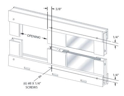
Slide the clear vinyl jamb seal [K] into the pivot jamb [L] and trim flush at both ends. The vinyl should be turned to trap water from the showerhead. Secure the vinyl with a small quantity of glue or caulk at each end or by carefully crimping the vinyl pocket.
