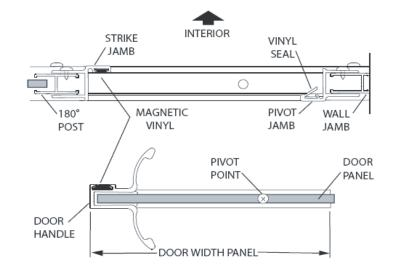
Snap the fillers [N] into the curb [A] and header [H] between the door jambs with the RAISED LIP TO THE EXTERIOR and the pivot holes toward the pivot jamb. Center the curb filler in the curb between the pivot and strike jamb (use masking tape to hold in position).
