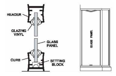
Carefully caulk the interior jamb-to-wall and curb-to-base joints. For appearance, you may wish to caulk the exterior joints as well. We recommend you wait twenty-four hours before the first shower to allow the caulking to cure properly.
