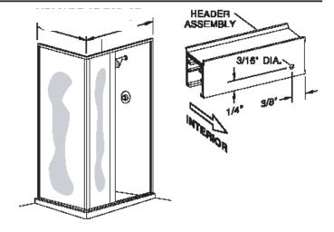
Press the header assembly [**D**] over the wall jambs [**E**] and the 90° post [**K**]. Check the posts for plumb. Adjust as required by varying the overlap of the header over the wall jambs. You may need to trim the ends of the header where it meets the wall. The minimum horizontal dimension for the door opening is the door panel width (see the graphic in Step #**9**) plus 1/2", maximum is the door panel width plus 1 3/4".
