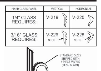
Cut four pieces of the smaller vinyl [JJ] 1" longer than the vertical opening (to prevent gapping from shrinkage) and trim the ends on a 45° angle. Using the masking tape guides, center the glass panel [J] in the frame. Cut four short (1" - 2") pieces of the small vinyl and press into the jamb and post on each side to hold the glass temporarily.
