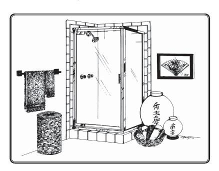
**MAINTENANCE:** Two primary materials are used to manufacture your new Aquatic enclosure; tempered glass and anodized aluminum. To assure a long lasting finish on the enclosure, wipe it down with a towel after each use. Never use a scouring agent to clean the aluminum.
