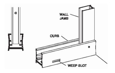
Wipe the shower walls and sill, curb assembly [A] and wall jambs [E] with a clean, dry cloth to remove any dust or debris. Apply a 1/4" bead of caulk along the inside of both of the pencil lines marked in Step #3. Carefully replace the curb in the exact position marked. Caulk the inside of the curb ends where they meet the wall. Caulk generously around the anchor plate [B], screws [C], and the inside of the mitered joints.
