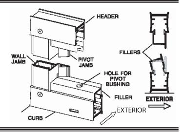
Pull the bottom end of the pivot jamb [M] tight to the curb filler [P] and plumb the jamb. Drill two 1/8" holes thru the pivot jamb and into the wall jamb [E] 3/8" to 3/4" from the wall and approximately 1/4" from the ends of the jamb. Drill a third hole centered between the first two, then enlarge the outer holes with a 3/16" drill for clearance on the self-tapping screws. Attach the pivot jamb permanently with three #8 x 1/4" truss head screws [C].
