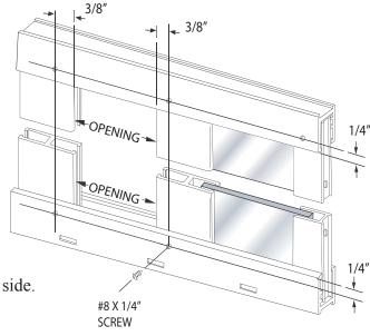
Slide the strike jamb [I] over the 180° post opposite the desired hinge side. Use a piece of tape to temporarily hold in place.
