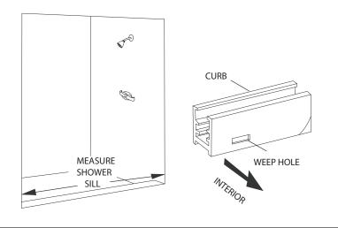
Place one wall jamb [D] into the curb against the wall. Using a level, plumb the wall jamb and mark the hole locations on the wall with a pencil. Repeat this step for the other wall jamb. Remove all parts and drill the holes.
