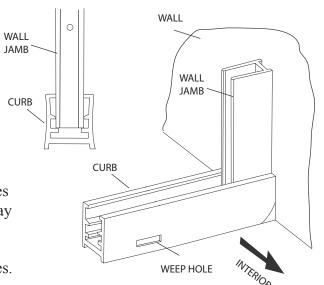
Wipe the shower walls, sill, curb & wall jambs with a clean, dry cloth to remove any dust or debris. Apply a 1/4" bead of silicone along the inside of the pencil lines that were marked in Step #2. Carefully place the curb on the sill, over top the silicone, in the position marked.
