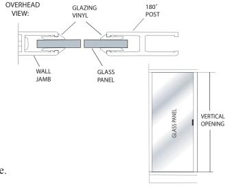
15 Cut eight (8) pieces of the horizontal vinyl [V] 1/2" longer than the horizontal opening. Cut both ends of the vinyl with a back mitre so that they sit tight against the face of the vertical vinyl. (see illustration)
