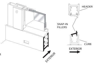
Question Center the door in the opening by sliding the hinge jamb over the 180° post until the hinge jamb is **plumb** and the space between the door glass and header is **even** from hinge side to strike side. Drill two 1/8" holes thru the hinge jamb and into the 180° post approximately 1" from the ends of the jambs at the top and bottom and approximately 3/8" from the edge of the open side of the hinge jamb.
