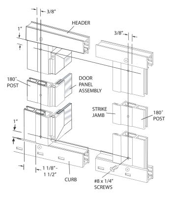
Drill and attach the strike jamb in the same manner as the hinge jamb.
