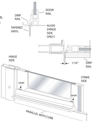
Hold the drip rail in place and adjust the drip vinyl by sliding it left or right until it there is a 1/16" gap between the bottom of the vinyl and the top of the snap-in-filler. Trim the vinyl flush with the hinge side of the rail and 3/8" longer on the strike side. Notch the top of the drip vinyl. (see illustration)
