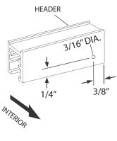
Slide the header over the wall jambs and 180° posts. Plumb one of the 180° posts, making sure to maintain the proper coverage over the glass panels of 1/4" to 3/4" as described in Step # 5. Mark its' location on the header and curb with a light pencil mark or a piece of tape. Repeat this step for the other 180° post.
