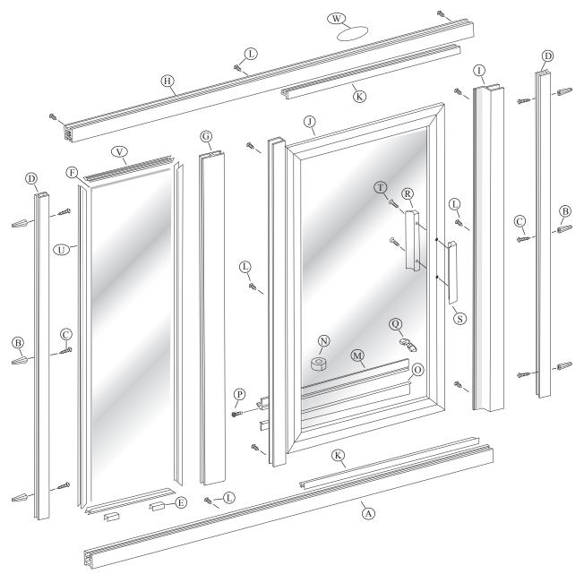
The Aquatic Continuous Hinge Shower Enclosure is completely reversible and may be installed hinge right or hinge left. For maximum leak protection, the hinge side should be opposite the shower head. Using the illustration, determine the proper hinge side for the door. This instruction sheet depicts a hinge-right installation. Careful as to not follow the illustrations exactly.
