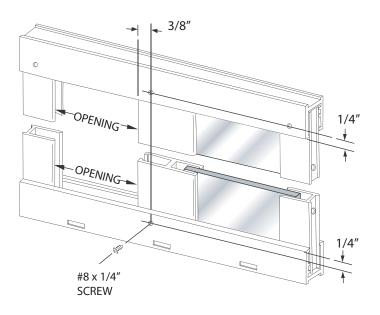
Slide the strike jamb [I] over the 180° post or the wall jamb, depending on hinge orientation. Use a piece of tape to temporarily hold in place.
