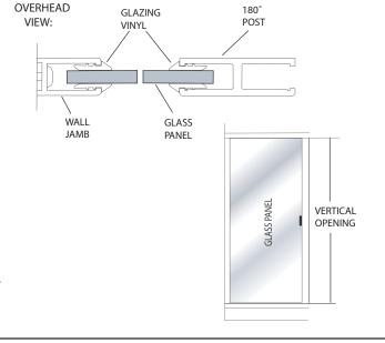
15 Cut four (4) pieces of the horizontal vinyl [V] 1/2" longer than the horizontal opening. Cut both ends of the vinyl with a back mitre so that they sit tight against the face of the vertical vinyl. (see illustration)
