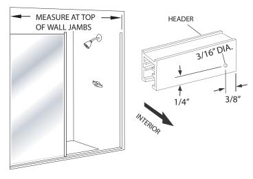
Slide the header over the wall jambs and 180° post. Plumb the 180° post, making sure to maintain the proper coverage over the glass panel of 1/4" to 3/4" as described in Step # 5. Mark its' location on the header and curb with a light pencil mark or a piece of tape.
