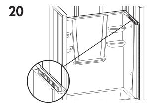
Check for level. Shim if necessary.
