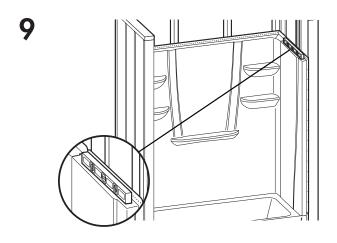
Check for level. Shim if necessary.
