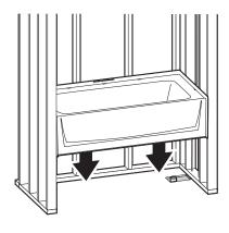
Lift and place the base into framing.
