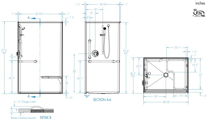
FEATURES Dimensional Tolerance ± %". Dimensions needed for site preparation should be measured from the unit. Aquatic assumes no responsibility for preparatory work.
