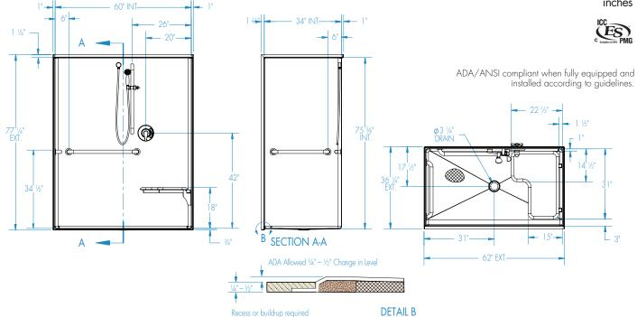
**FEATURES** Dimensional Tolerance ± %". Dimensions needed for site preparation should be measured from the unit. Aquatic assumes no responsibility for preparatory work.
