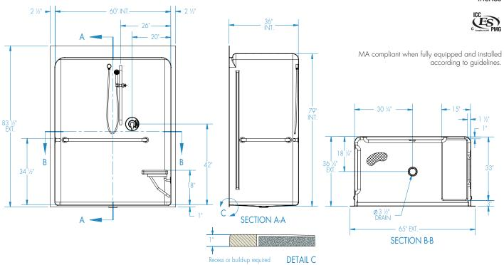
FEATURES lbs (kg) Dimensional Tolerance ± %". Dimensions needed for site preparation should be measured from the unit. Aquatic assumes no responsibility for preparatory work
