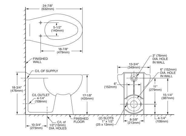
NOTES: \* VARIABLE — CHECK WITH MANUFACTURER OF FLUSHVALVE FOR PROPER ROUGH-IN DIMENSIONS. WASTE OUTLET SEAL RING MUST BE NEOPRENE OR GRAPHITE-FELT (WAX RING NOT RECOMMENDED). TO COMPLY WITH AREA CODE GOVERNING THE HEIGHT OF VACUUM BREAKER ON FLUSH VALVE, THE PLUMBER MUST VERIFY DIMENSIONS SHOWN FOR SUPPLY ROUGHING. FLUSH VALVE NOT INCLUDED AND MUST BE ORDERED SEPARATELY.
