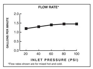
1.5 gpm/5.7 L/min. FLOW RATE
