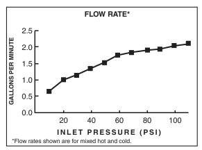
1.8gpm/6.8L/min. FLOW RATE
