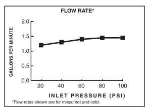
1.5 gpm/5.7 L/min. FLOW RATE
