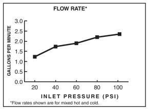
2.2gpm/8.3L/min. FLOW RATE
