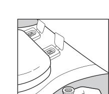
With the plastic bolts installed, thread the winged plastic nuts on to the bolts.
