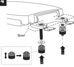
When opened, nuts can slip over threads for rapid installation.
