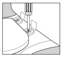
Tighten the bolts using a screwdriver.
