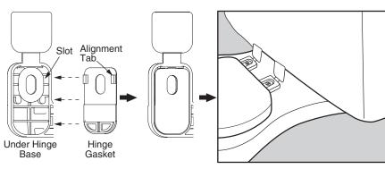
Attach hinge gaskets to bottom of hinge base. Make sure alignment tabs on hinge gaskets match the slots under the hinge base.
