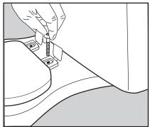
When the seat is properly aligned with the front edge of the bowl, slip the bolt through the washer and the bowl bolt holes.
