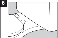
The hinge cap covers are designed to snap lock on to the hinge. Position the hinge covers and push down on the cover.
