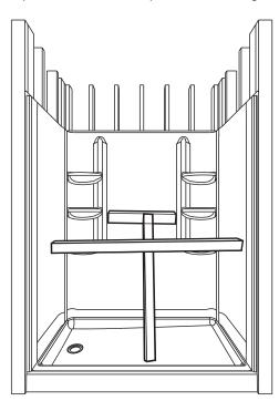
When installing greenboard, position drywall screws above the top nailing flange. If you choose to screw through the nailing flange, you MUST drill clearance holes in the flange to avoid cracking/damaging the flange.
