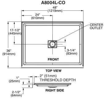
Ensure that the floor and stud walls are square and plumb on a level floor as shown in Figure A. Provide a 5" x 5" (127 x127mm) opening in the floor for the drain and refer to the product rough-in for actual drain location. Draw a line 3-1/2" (89mm) [model A8003L-LHO/A8003L-RHO draw a line 4" (102mm)] above the level subfloor on the wall studs at each side of the opening.
