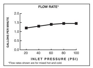
1.5 gpm/5.7 L/min. FLOW RATE
