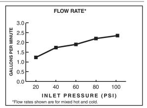
2.2 gpm/8.3 L/min. FLOW RATE
