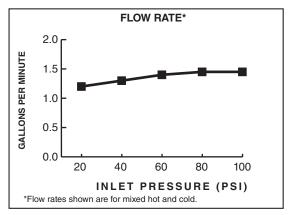
1.5 gpm/5.7 L/min. FLOW RATE
