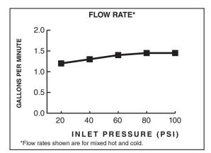
1.5 gpm/5.7 L/min. FLOW RATE
