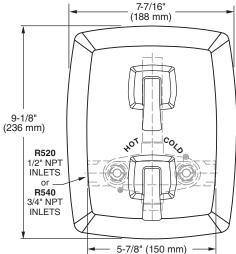
NOTE: FITTING MUST BE INSTALLED WITH VOLUME CONTROL ON TOP.
